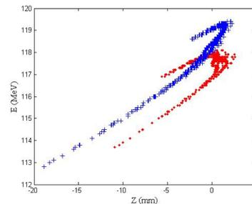
Figure 9: The result from MathCAD after the INFN-Frascati chicane with changing the phase by -20 degree in girder 15 from crest ( $\sigma=1.47$ mm) and without changing the phase (+) ( $\sigma=2.43$ mm). Input is from MathCAD.
