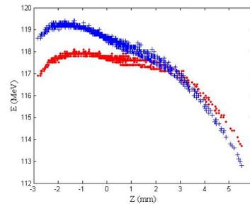
Figure 8: The result from MathCAD before the INFN-Frascati chicane with changing the phase by -20 degree in girder 15 from crest and without changing the phase (+). For both:  $\sigma=1.62$  mm. Input is from MathCAD.
