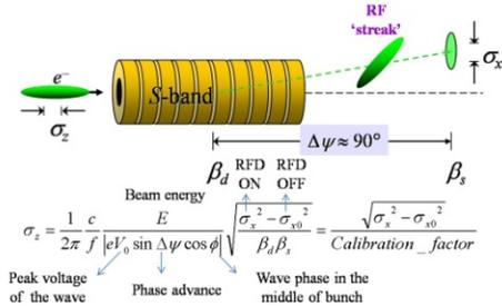
Figure 10: Using RF deflector for bunch length measurement [4]. f=1.5 GHz.
