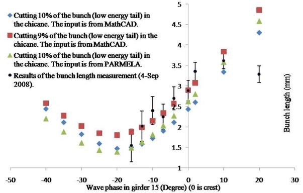
Figure 13: The result of bunch length measurement by RF deflector and the result of different simulations.
