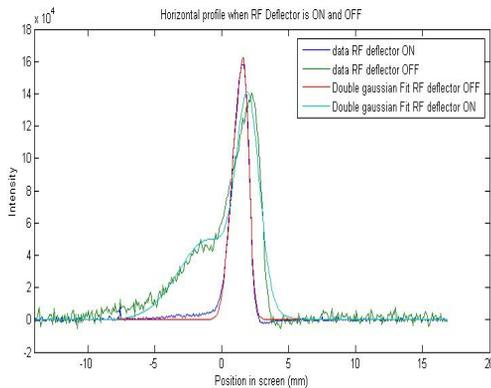
Figure 12: This shows the horizontal profile on screen when the RF deflector is ON and when it is OFF. ( $\sigma > \sigma_0$ ).
