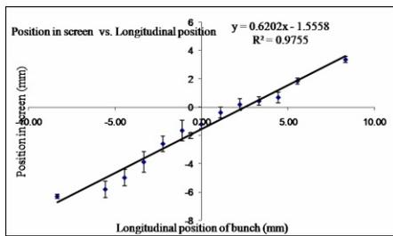
Figure 11: The method for finding the calibration factor that shows the relation between the screen position unit and the longitudinal position unit.
