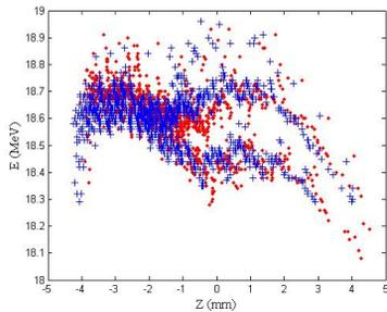
Figure 4: The result from MathCAD (no wake field) and PARMELA (+) after chicane starting from the end of the injector. Input is from PARMELA.
