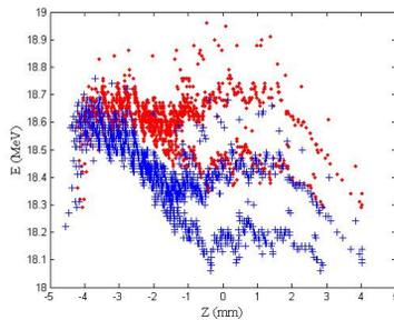
Figure 5: The result from the MathCAD after the chicane with wake field (+) (input for the MathCAD) and without wake field.
