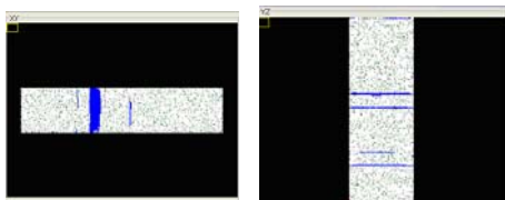
Figure 2: Multipactor discharge region in narrow rectangular waveguide.
