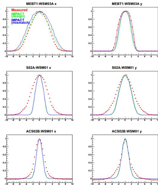
Figure 5: Horizontal (left) and vertical (right) beam profiles at MEBT1 (top), SDTL entrance (middle), and SDTL exit (bottom). Red dots show measured data with WS's. Blue lines show IMPACT calculations with the initial beam parameters from fit at MEBT1. Green lines show IMPACT calculations mismatched at the entrance of DTL1 by deviating initial Twiss parameters
