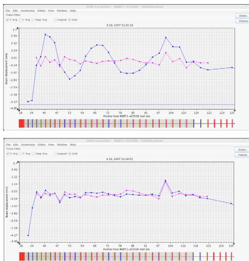
Figure 6: Horizontal orbit positions as a function of a distance at SDTL before correction (top) and after correction (bottom). Blue lines show measured beam positions, and pink lines show predicted positions.
