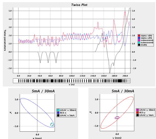
Figure 4: Top: Horizontal (red line) and vertical (blue line) envelopes fit to profile widths (points) and dispersions (m) (black line) calculated by the model at different sets of QM field for "Half-matched" setting at 5 mA. Bottom: Horizontal (left) and vertical (right) phase ellipses of LINAC beam at the injection point at 5 mA and 30 mA with "Half-matched" setting compared to RCS phase ellipse.
