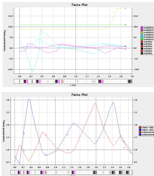
Figure 3: Top: measured transverse emittance and Twiss parameters with the double-slit emittance monitor at MEBT1 bend line. Bottom: measured profile widths with wire scanners at MEBT1. The curves show simultaneous fit with entrance transverse and longitudinal emittance and Twiss parameters.
