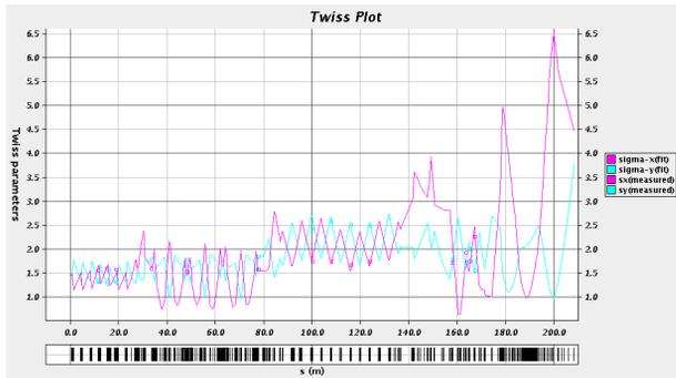
Figure 2: Horizontal (pink) and vertical (blue) 1  $\sigma$  beam widths [mm] at L3BT fit to XAL model at 30 mA.
