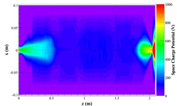
Figure 2: Two dimension projection in (z0x) plane of a space charge potential map.
