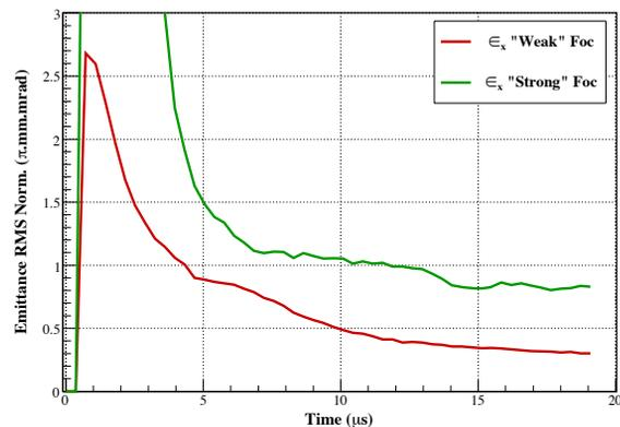
Figure 3: Emittance evolution as a function of time, for the two type focalisation conditions. The simulation starts at time  $t=0$ .
