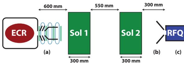
Figure 1: Scheme of the IFMIF-EVEDA LEBT. (a): ECR extraction system - (b): RFQ injection cone - (c): first RFQ segment.
