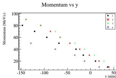
Figure 5: Momentum as a function of vertical position for an on-axis, parallel muon beam with a momentum range of 10–150  $MeV$ .
