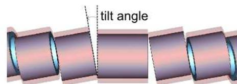
Figure 2: Drawing of the bent, tilted muon transport channel of the COMET beamline showing the tilt used to produce the vertical dipole field. The tilt angle shown here is exaggerated as the angle used in the simulations is  $1.43^\circ$ .
