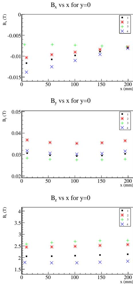
Figure 3: Results of the G4Beamline simulation. The plots show the  $B_x, B_y$  and  $B_z$  components as a function of  $x$  for the different powering schemes described in Table 1.
