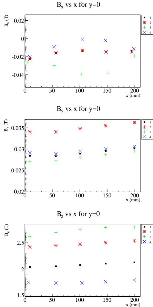
Figure 4: Results of the EM Studio simulation. The plots show the  $B_x, B_y$  and  $B_z$  components as a function of  $x$  for the different powering schemes described in Table 1.
