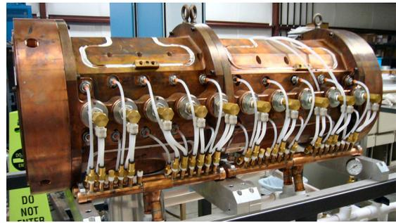
Figure 5: RFI cooling circuits.
