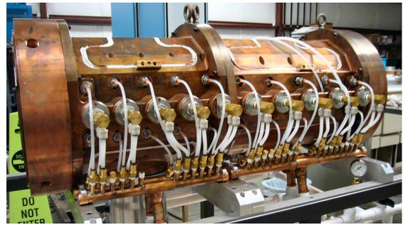
Figure 5: RFI cooling circuits.
