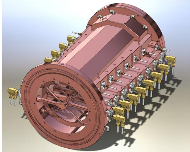
Figure 3: Multi-cell RFI linac structure.
