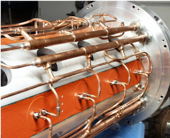
Figure 4: RFQ cooling circuits.
