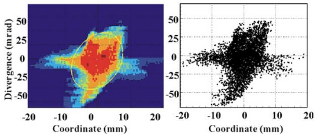
Figure 4: Measured  $^{12}\text{C}^{4+}$  emittance at the RFQ entrance (left) and generated particle distribution to be used for simulation.
