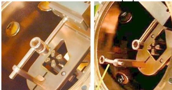
Figure 8: Rebuncher structure as mounted for operation (left) and in a dummy position to measure the output energy of the RFQ itself (right).
