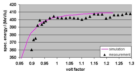
Figure 11: The RFQ energy scan with the rebuncher in the dummy position (blue) and the theory curve (red).
