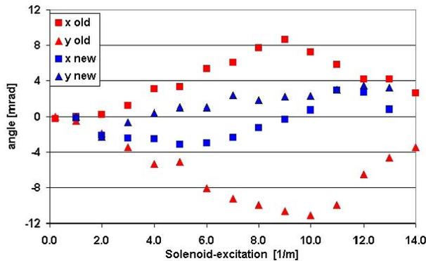
Figure 3: Steering of the beam behind the old and new Solenoids depending on their field strengths.
