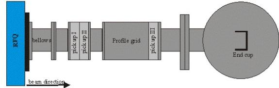
Figure 10: A photo of the diagnostics test bench as currently installed at Risø for RFQ energy measurements (top) and a schematic drawing (bottom).
