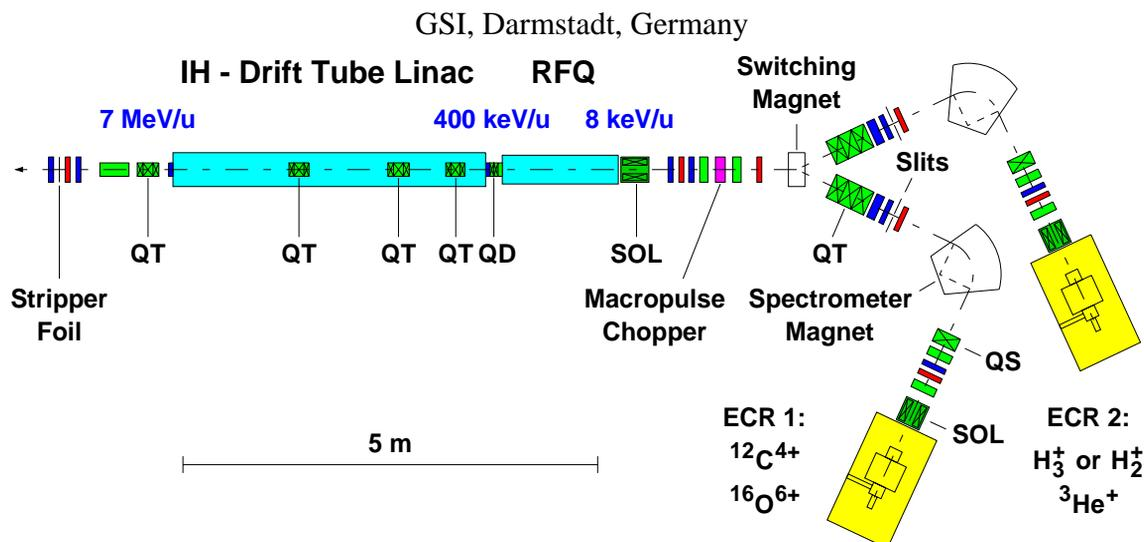
Figure 1: Layout of the Injector Linac [1]. QS = Quadrupole singlet, QT = Quadrupole triplet, SOL = solenoid, magnetic focusing and steering magnets (green), profile grids and the tantalum screen (red), and the beam current monitors (blue).
