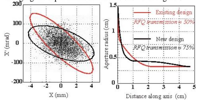
Figure 5: Dynamion simulation of the transmission improvement through the old and the new input radial matcher design using the particle distributions generated from the measured emittances (Figure 4).
