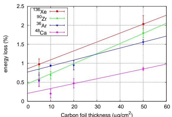
Figure 6: Beam energy loss as a function of the target thickness. Fit by Eq. 2.
