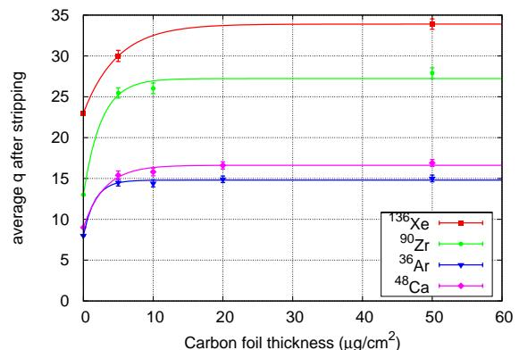
Figure 5: Beam average charge  $\bar{q} = \sum_q P(q)$  as a function of target thickness. Fit by Eq. 1.
