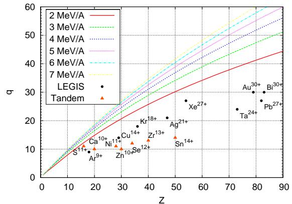
Figure 2: Most probable charge state from stripper as function of Z and energy compared to some examples of available ions out of LNL Tandem injector or foreseen for the new LEGnaro ecrIS (LEGIS).
