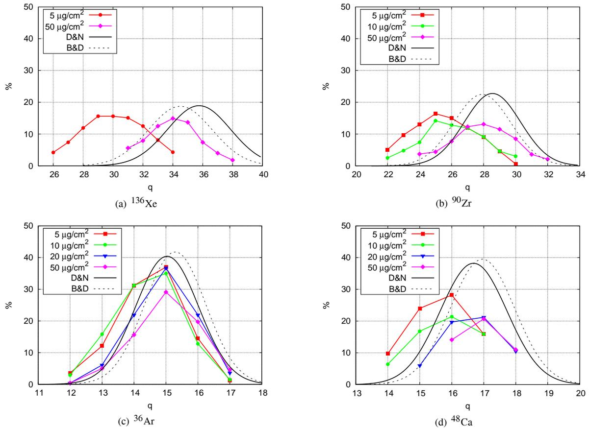
Figure 4: Stripping probability as function of the target thickness. Semi-empirical formulas predictions are added as comparison. The data are normalized on the beam current before stripping.
