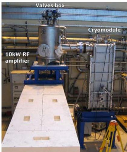
Figure 4: qualification type A cryomodule ( $\beta=0.07$ ).
