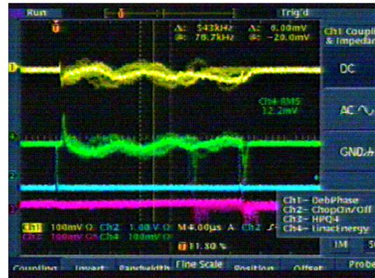
Figure 1: Velocity meter scope traces.
