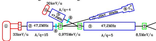
Figure 1: The structural scheme of the MILAC.
