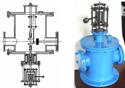
Figure 5: Chamber for investigations of plastic properties of structural materials exposed to the ion beam.
