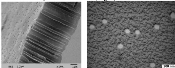
Figure 4: Pores at the cross section and the surface track-etched membrane.
