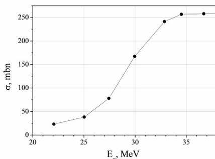
Figure 6: The function for excitation of  $^{16}\text{O}(\alpha, pn)^{18}\text{F}$ .
