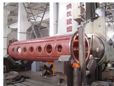
Figure 1: The first module tank is under fine machining after copper electroform.
