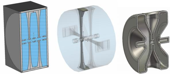
Figure 1: RT CH model consisting of background PEC, cavity components and vacuum filling is on the left. In the center a separate half of spoke is shown. Model of single spoke superconducting cavity SSR is on the right.
