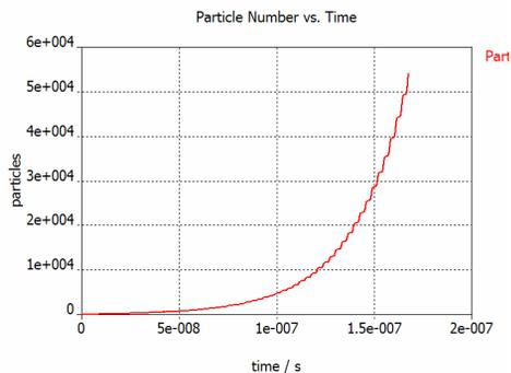
Figure 3: Exponential growth of particle number in a cavity when MP conditions are fulfilled.
