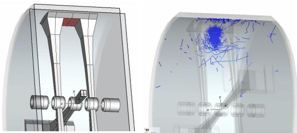
Figure 2: Initial electron source and particle trajectories in CH1 after 40 RF periods (crashed particles are not shown).
