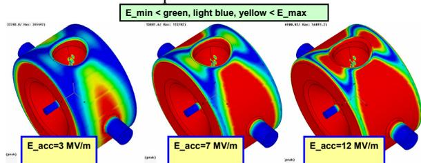
Figure 5: Electric surface field distribution at different accelerating gradients.
