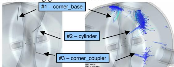
Figure 7: The initial electron sources in different locations.
