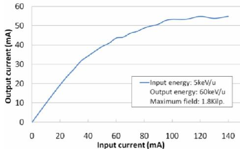
Figure 3: Output current versus the input current per beam channel.
