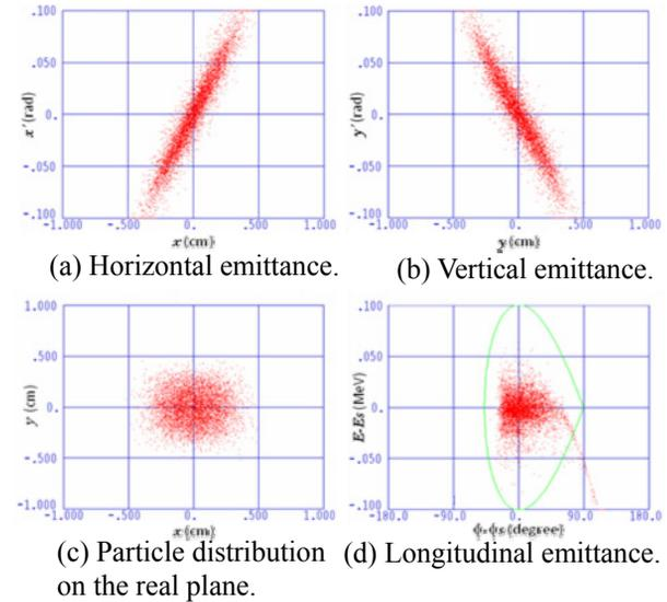
Figure 2: Beam profile at the end of the 4-rod.
