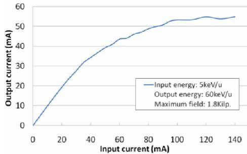
Figure 3: Output current versus the input current per beam channel.
