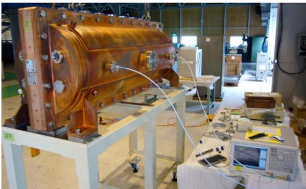
Figure 5: Low power RF measurement of the 2-beam type IH-RFQ cavity.
