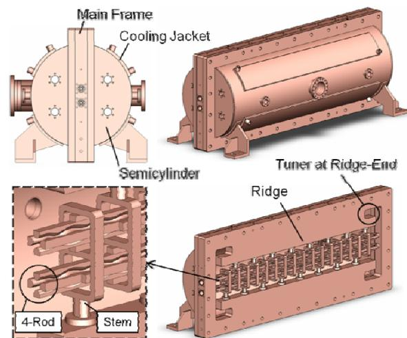
Figure 1: External appearance of the 2-beam type IH-RFQ.
