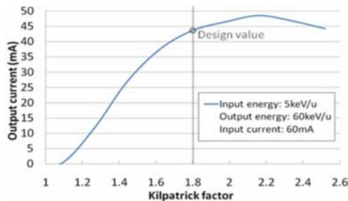
Figure 4: Output current per beam channel versus Kilpatrick factor.
