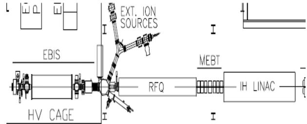
Figure 1: Layout of the EBIS Linac at BNL.
