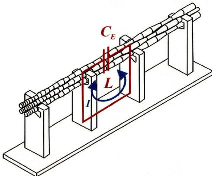
Figure 3: Basic cell of the 4-Rod RFQ structure.
