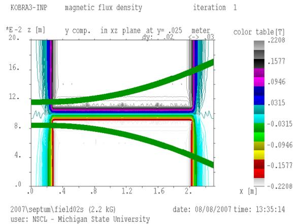
Figure 7: The path of the two separated bunches and the magnetic field distribution in the septum magnet.
