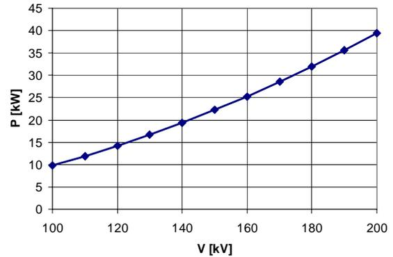
Figure 5: RF power losses in the structure vs. inter-plate voltage.
