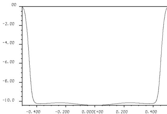
Figure 4: Transverse electric field profile in the RF kicker along the beam axis.
