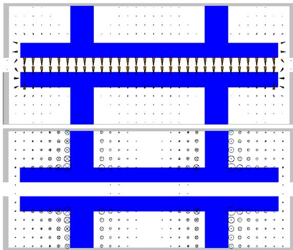
Figure 3: Electric (top) and magnetic (bottom) field distribution in a central vertical cross-section along the beam axis of the RF kicker structure.
