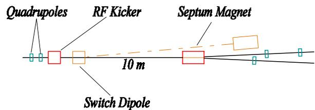
Figure 1: Layout of a proposed FRIB BSY system.
