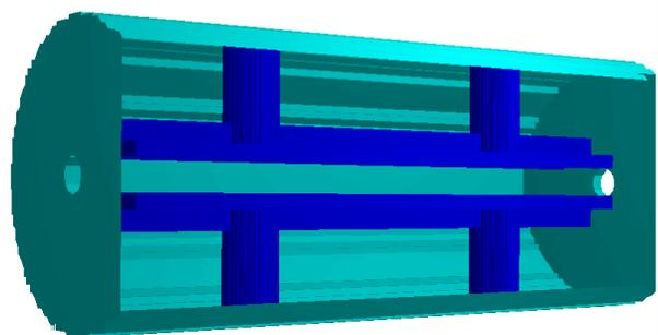
Figure 2: Three-dimensional view of the RF kicker.
