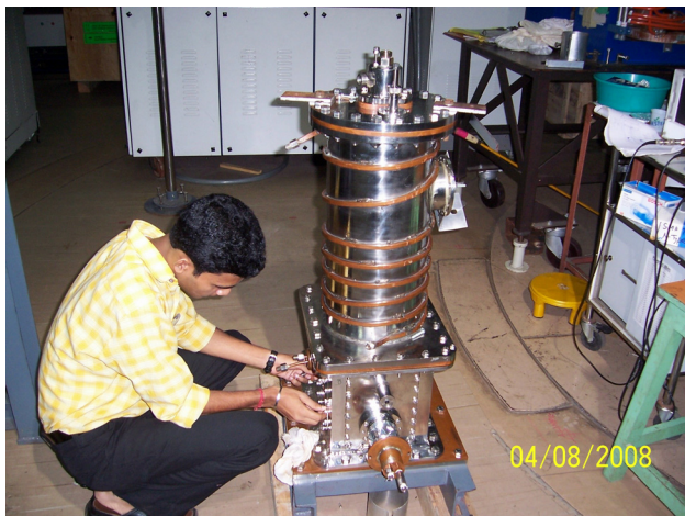
Figure 4: The Re-buncher during assembly.
