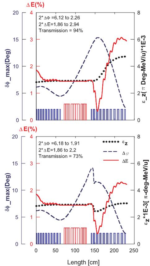
Figure 1: A typical tune through two LINAC cavities showing the variation of rms energy width, phase width and longitudinal emittance growth.
