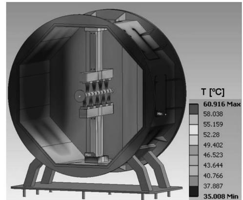
Figure 2: Temperature profile of LINAC-2 calculated using ANSYS.
