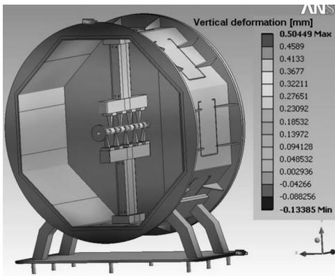
Figure 3: Structural deformation of LINAC-2 calculated using ANSYS.
