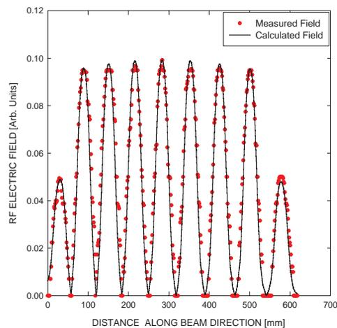
Figure 5: Results of bead perturbation measurement of LINAC-1.
