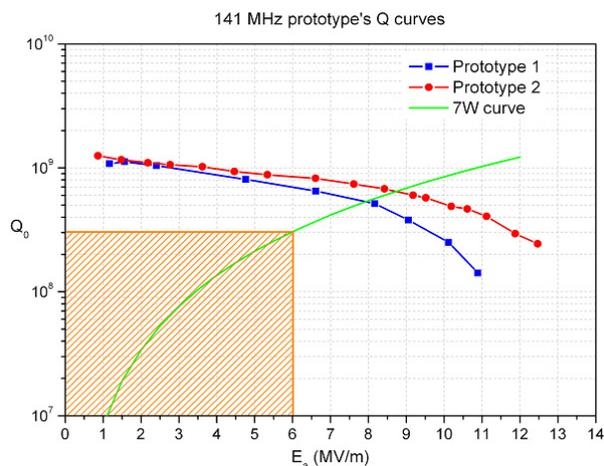
Figure 3: Characterization curves of the two 141 MHz QWR cavities.
