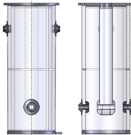
Figure 2: The 141.44MHz rf cavity for Phase II.
