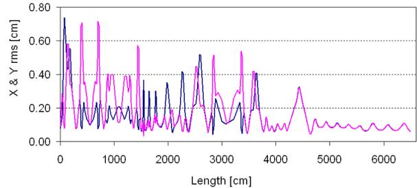
Figure 5: The x (magenta) and y (blue) beam envelopes from RFQ2 to the end of the ISAC-II SC-linac.
