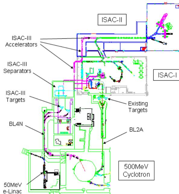
Figure 1: The TRIUMF site including the cyclotron, ISAC-I and ISAC-II and the proposed ISAC-III (ARIEL) facility. BL2A is the present proton line and the BL4N tunnel is proposed for the new ISAC-III driver beams.
