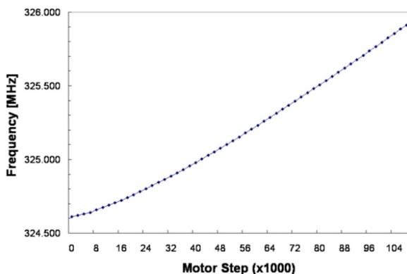
Figure 6: Cavity resonant frequency versus tuner position.
