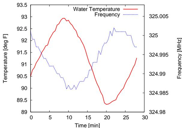
Figure 3: Cavity resonant frequency measured against coolant temperature.
