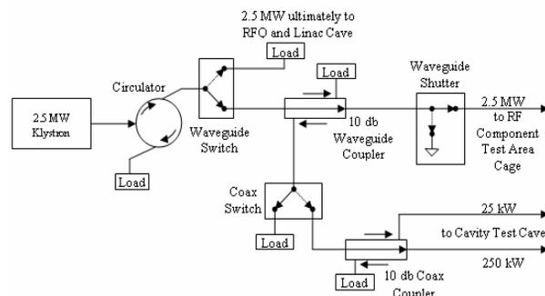
Figure 2: RF power and distribution system diagram.
