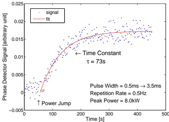
Figure 5: Dynamic measurement of cavity resonant response to RF power.
