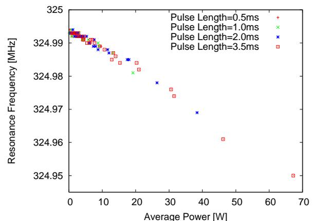
Figure 4: Cavity resonant response to RF power.
