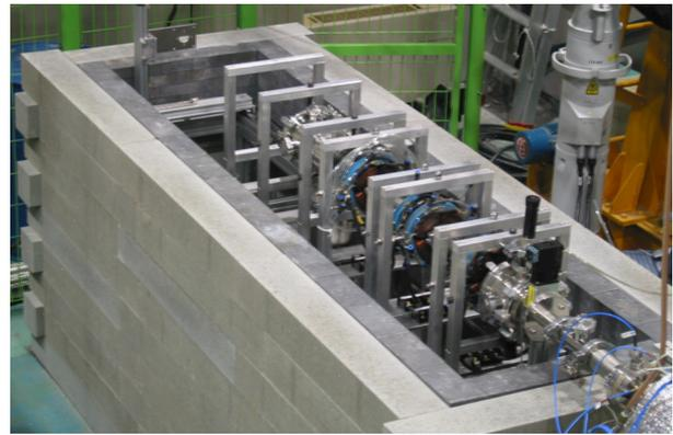
Figure 2: 20MeV proton beam target station.
