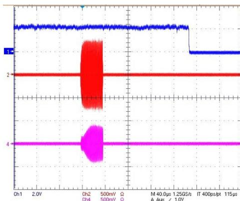
Figure 5: Beam signal of PEPF 20MeV linac (Ch 1: proton injector, Ch 2: RFQ, Ch 4: DTL).
