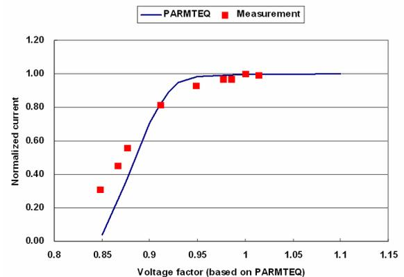
Figure 3: RFQ transmission rate depending on the vane voltage.
