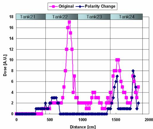
Figure 4: Beam loss distribution along the DTL (original: purple, after polarity change: blue).
