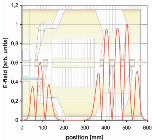
Figure 4: Field distribution on beam axis along IH-DTL.
