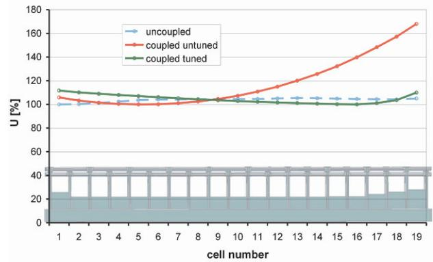
Figure 3: Simulation of the field distribution on RFQ-axis. The different height of tuning plates is indicated for the coupled and tuned case. The aperture is held constant here.
