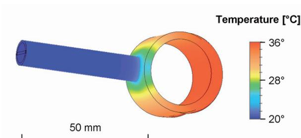
Figure 5: Simulation of thermal load on an IH-drifttube.
