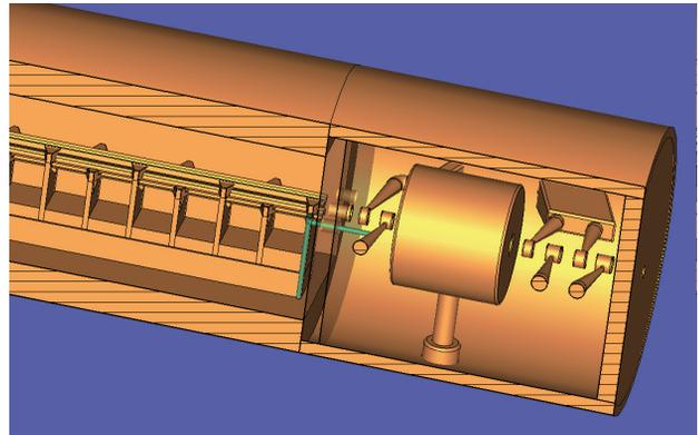
Figure 1: The coupled 4-rod-RFQ-IH-DTL structure. The coupling bridges are colored in green.
