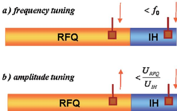
Figure 2: Tuning of frequency and amplitude during operation. Both tuners are acting inductively.
