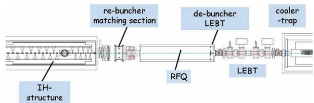
Figure 7: The RFQ section of the HITRAP decelerator.
