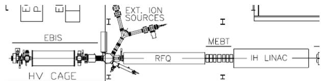
Figure 9: Layout of the EBIS Linac at BNL.
