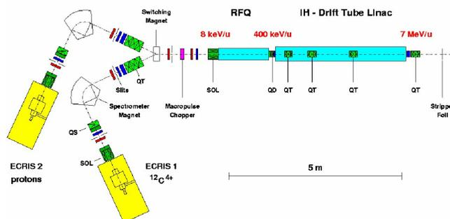
Figure 5: Layout of the HICAT injector.
