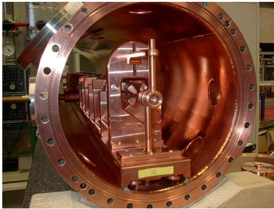
Figure 6: View of the HIT-RFQ with rebunching section.
