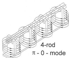
Figure 3: Scheme of a 4-Rod-RFQ resonator insert.
