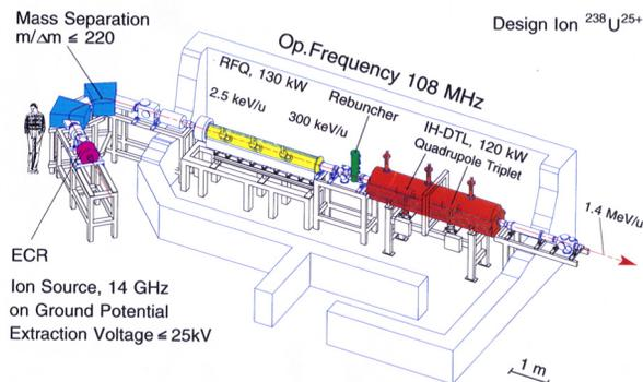
Figure 4: The HLI-injector of GSI.
