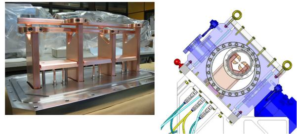
Figure 11: Prototype high power RFQ insert and tank.
