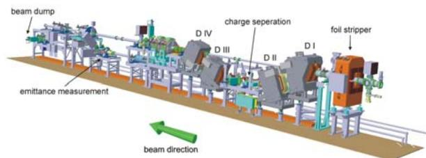
Figure 6: New Charge state separator system, integrated in the TK comprising the foil stripper, the four 35°-Dipole magnets (DI - DIV), and a beam diagnostics bench.
