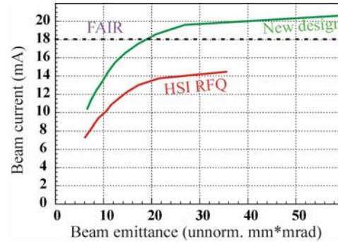
Figure 2: Beam current inside a given emittance at RFQ-output for the existing (red) and the new design (green).
