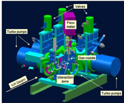
Figure 4: New gas stripper box.
