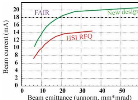
Figure 2: Beam current inside a given emittance at RFQ-output for the existing (red) and the new design (green).
