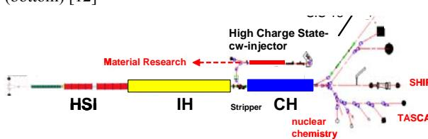
Figure 11: Conceptual layout of a multipurpose high intensity heavy ion linac at GSI [13]
