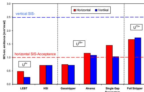
Figure 8: High current beam emittance measured during the measurement campaign in June 2008.
