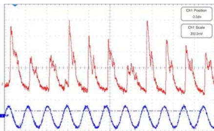
Figure 10: Bunch measurement of a 4 MeV/u  $^{20}\text{Ne}^{10+}$ - beam with the diamond detector (top) and 108 MHz reference signal (bottom) [12]
