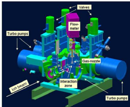
Figure 4: New gas stripper box.
