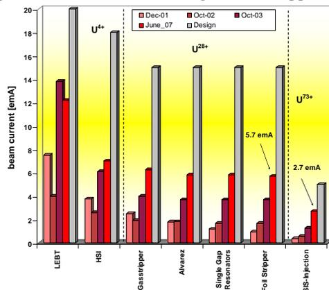
Figure 7: Improvement of the UNILAC-uranium beam intensities during the last three years.
