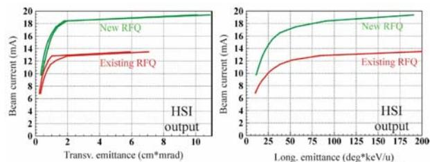
Figure 3: Beam current inside a given transverse (left) and longitudinal (right) emittance at HSI-output for the existing (red) and the new design (green). [6]
