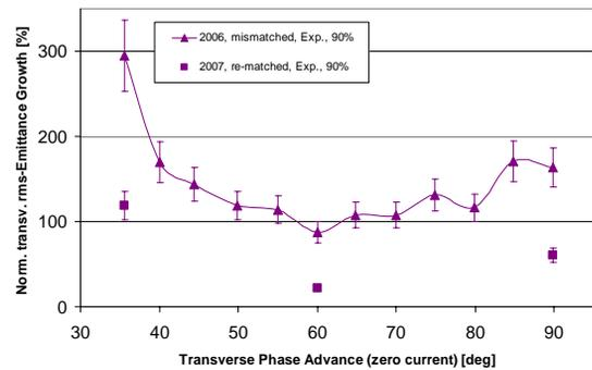
Figure 5: Measured transverse emittance growth as function of the phase advance [9]
