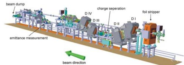
Figure 6: New Charge state separator system, integrated in the TK comprising the foil stripper, the four  $35^\circ$ -Dipole magnets (DI - DIV), and a beam diagnostics bench.
