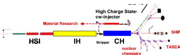
Figure 11: Conceptual layout of a multipurpose high intensity heavy ion linac at GSI [13]
