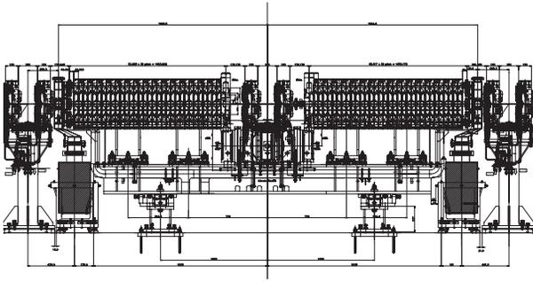
Figure 5: The layout of an ACS module. Two ACS tanks are connected with a bridge coupler. Quadrupole doublets are placed between ACS tanks to provide the transverse focusing.
