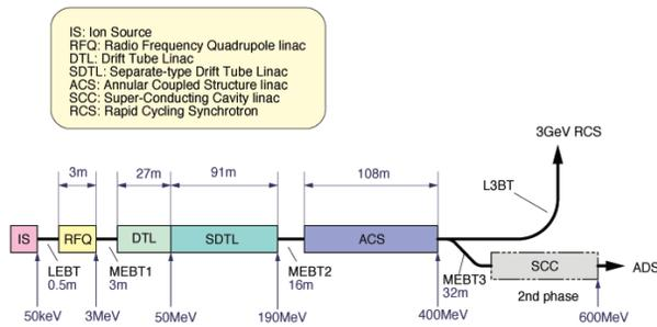
Figure 2: Schematic layout of J-PARC linac.
