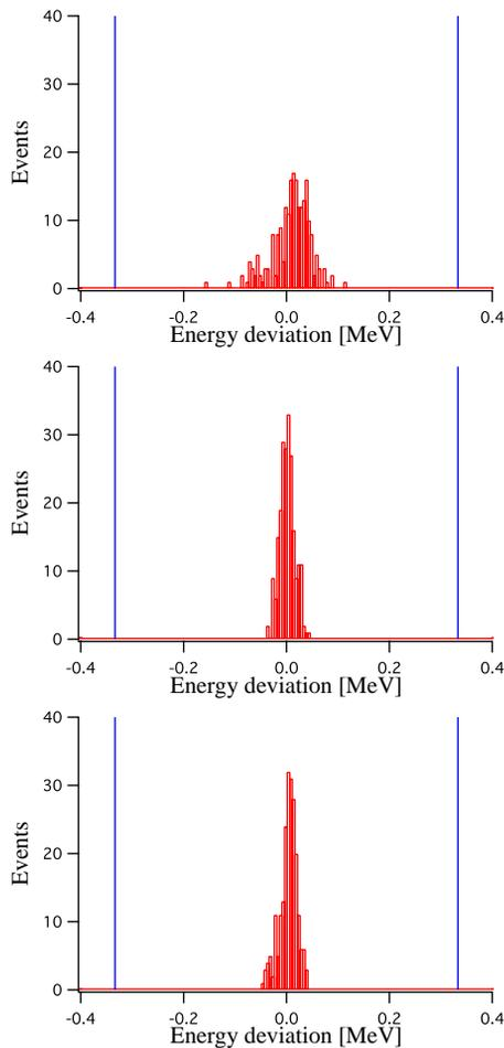
Figure 3: Energy jitter at the SDTL exit (top), the first debuncher exit (middle), and the second debuncher exit (bottom). The blue vertical lines show the specification of  $\pm 0.1$  % in momentum.
