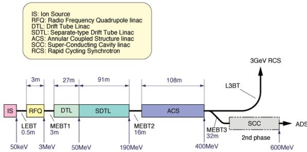
Figure 2: Schematic layout of J-PARC linac.
