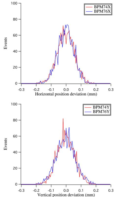
Figure 4: Beam position jitter for the last two BPM's in L3BT. Top: horizontal, bottom: vertical.
