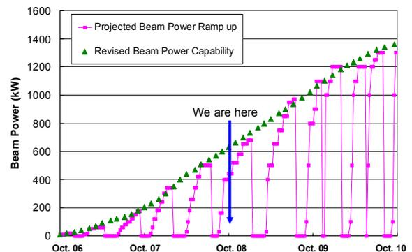
Figure 8: SNS beam power ramp-up history and plan.
