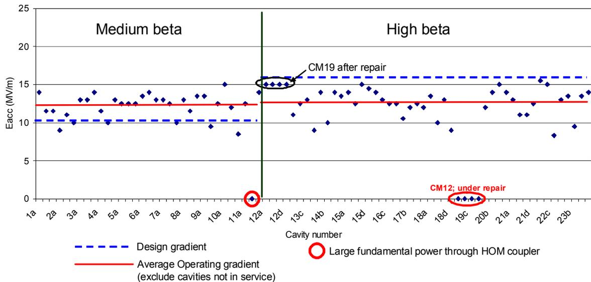
Figure 2: Operating setpoints of SCL SRF cavities at 60 Hz for the neutron production in 2008.
