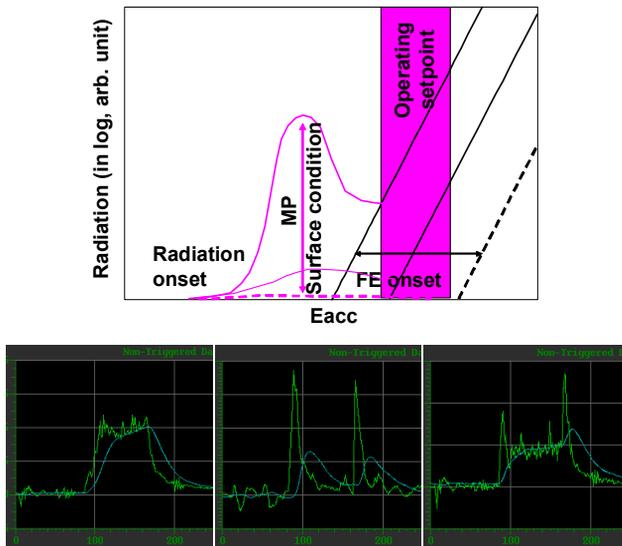
Figure 7: SNS SRF cavity operating regime at 60 Hz and radiation waveforms from RF operations depends on contents of electron activities in a cavity.
