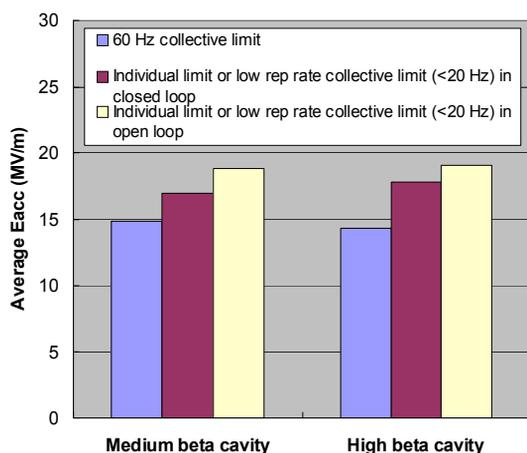
Figure 4: Comparisons of average limiting gradients at 60 Hz collective, individual (or low rep rate collective) in closed loop and that in open loop.
