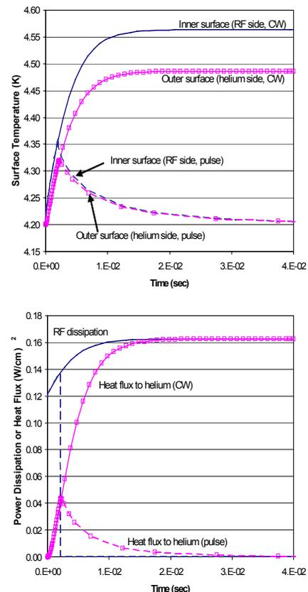
Figure 3: Comparisons of thermal parameters between CW and pulsed operations. Both cases are stable. (solid line; CW operation, dashed line; pulsed operation, lines with symbols; for surface at helium side, lines without symbols; for surface at RF side).
