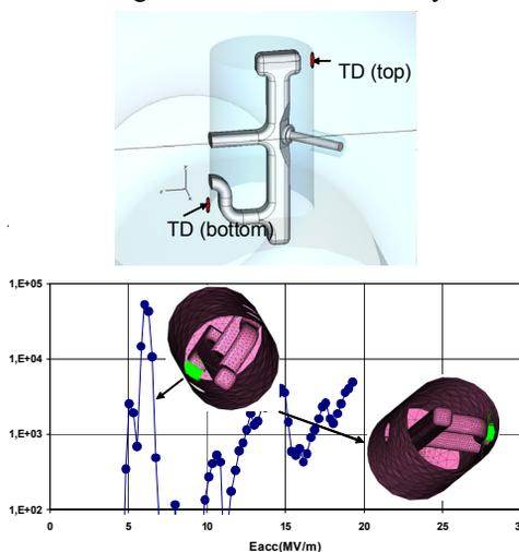
Figure 5: Thermal diodes locations of the 19b after removing the feedthrough (top). Multipacting simulation of the SNS high beta cavity HOM coupler [7] (bottom).
