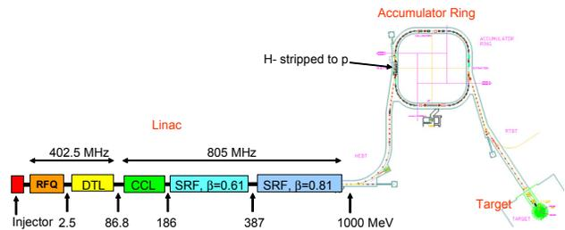
Figure 1: Layout of the SNS accelerator system.
