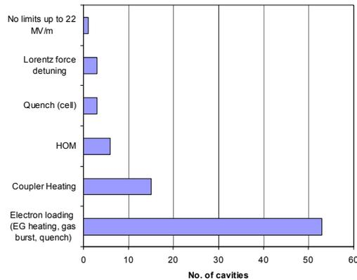
Figure 6: Statistics of limiting factors at 60 Hz collective condition.
