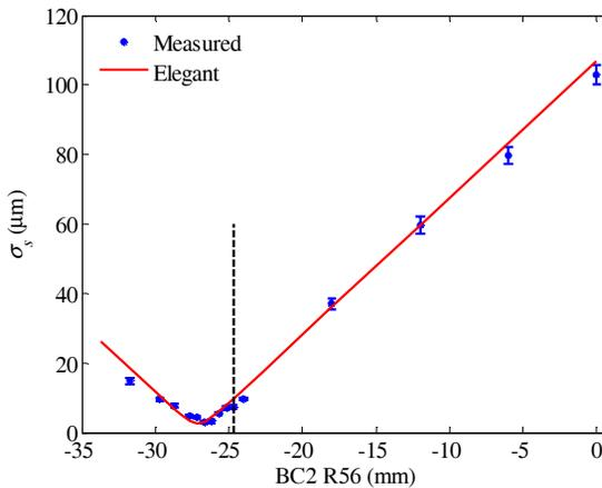
Figure 8: Bunch length after BC2 vs.  $R_{56}$  of the bunch compressor. The black line indicates the normal operating point at -24.7 mm and the red arrow the minimum bunch length.
