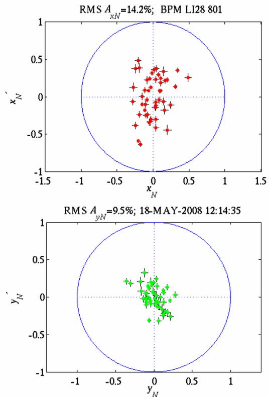
Figure 10: Shot to shot beam position and angle near the end of the linac in units normalized to the transverse beam phase space.
