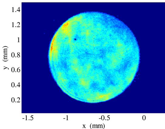
Figure 2: Laser distribution on the virtual cathode.
