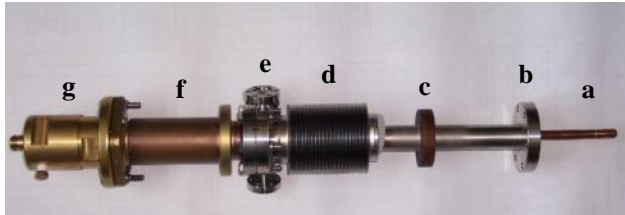
Figure 1: Assembled fundamental power coupler: (a) vacuum side inner conductor, (b) vacuum side outer conductor, (c) 77 K intercept, (d) bellows, (e) diagnostic ports, (f) air side outer conductor, (g) adapter to type N.
