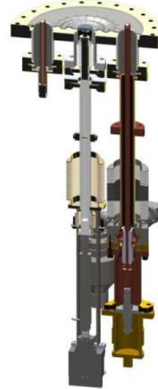
Figure 5: Power coupler and tuner assembly.
