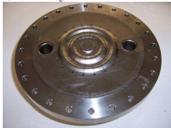
Figure 2: Niobium tuning plate with convolutions, slots, and RF ports.
