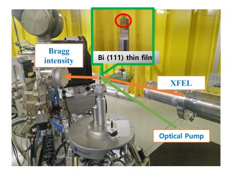
Bi(111) thin film (50 nm) on GaSb(111)/Si(111) X-ray: 6 keV X-ray size: ~ 60 x 60 um<sup>2</sup> Laser: 800 nm, 100 fs Detector: MPCCD 0.5M
