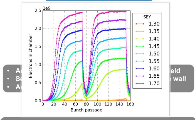
After the passage of several bunches, the electron distribution inside the chamber reaches a dynamic steady state (electron cloud)
