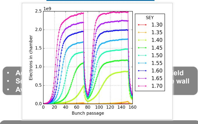
After the passage of several bunches, the electron distribution inside the chamber reaches a dynamic steady state (electron cloud)
