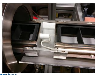
Dipole chamber cathode
