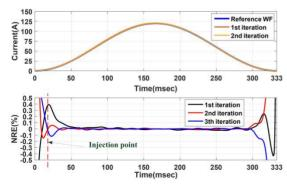
Figure 7: Reference and output waveform and NRE when waveform compensation is on.
