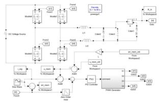
Figure 4: TPS quadruple magnet power model.
