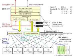
Figure 1: The control of TPS booster ring power supplies.
