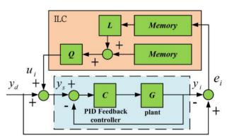
Figure 2: ILC feed forward with PID feedback control.
