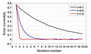
Figure 5: Tracking error current convergence curve with L set at 0.1, 0.5 and 1.
