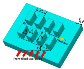
Figure 1: Schematic of a dual-grating structure illuminated by a PFT laser beam with a tilt angle of  $\gamma$ .  $\lambda_p$ , A, B, C, and H represent grating period, pillar width, pillar trench, vacuum channel gap and pillar height, respectively.  $A + B = \lambda_p$  is selected for all simulations.
