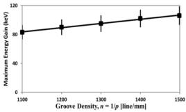
Figure 4: Numerically computed energy gain with different grating groove densities.
