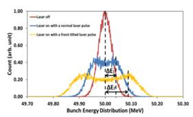
Figure 3: Bunch energy distribution for the cases of laser-off (red line), laser-on with a normal laser (blue line) and laser-on with a front-tilted laser (yellow line).
