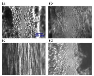
Figure 4: Images of the target rear surface. (a. 1.2  $\mu$ m thick aluminium target, (b. 2.5  $\mu$ m thick aluminium target, (c. 3  $\mu$ m thick titanium target, (d. 50 nm thick diamond-like carbon target, respectively. The scales of the figures are the same.
