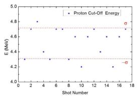
Figure 6: The shot-to-shot results of proton cut-off energy.
