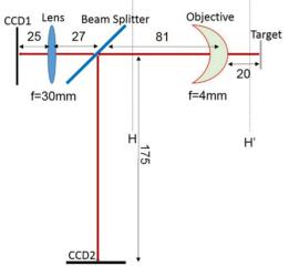
Figure 2: Schematic of the microscope system. The omitted unit is millimetre. Two different magnifications 10fold (CCD1) and 50-fold (CCD2) can be achieved simultaneously with the help of a beam splitter.
