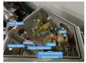
Figure 5: Target chamber for laser proton acceleration.
