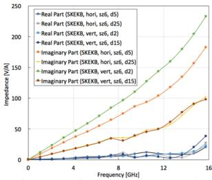
Figure 5: Real and imaginary parts of the impedances of collimators for a bunch length of 6 mm. *d* refers to an aperture.
