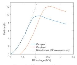
Figure 4: Lifetime vs. RF voltage.
