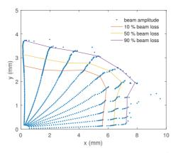
Figure 3: Dynamic aperture at the injection point following the installation of the DDBA cell.
