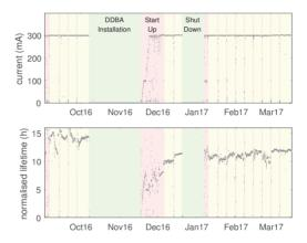
Figure 5: Stored beam current (top) and normalised lifetime (bottom) over the commissioning period. Shutdown periods are highlighted in green, machine development in red and user time is shown in yellow.
