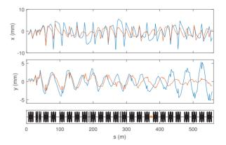
Figure 1: First-turn trajectory for the injected beam before (blue) and after (red) adjustment of the DDBA steerers.
