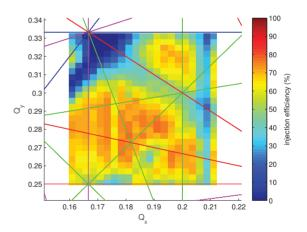
Figure 2: Injection efficiency vs. tune point with IDs closed
