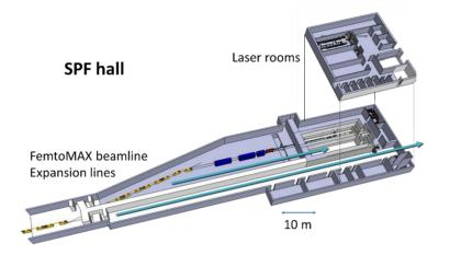
Figure 2: The existing SPF hall, the installed second bunch compressor and the FemtoMAX beamline. Blue arrows indicate tentative locations of the SXL.
