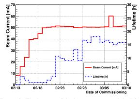
Figure 8: The history of the beam current and the lifetime. The displayed values of the beam current are the maximum ones, and those of the lifetime are the typical ones recorded for each day.
