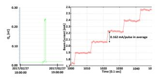
Figure 6: (Left) Charge amount detected at the end of Linac. (Right) Accumulated beam current of PF-AR ring.
