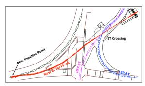
Figure 5: The injection section of the direct beam transport line for PF-AT.
