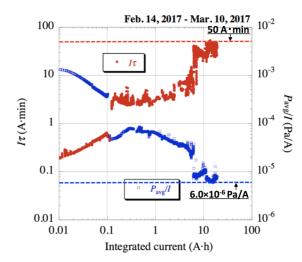
Figure 9: The state of the vacuum scrubbing of the PF-AR ring. Each dashed line indicates the goal estimated from the past results before the construction of the new BT.
