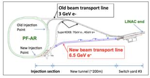
Figure 1: The schematic view of the old and the new direct beam transport line of PF-AR.
