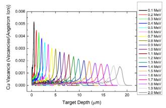
Figure 1: Depth distributions of vacancies in copper target correspond to normally incident proton beams with different energies from 100 keV to 2 MeV.
