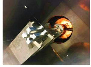
Figure 9: The bead- perturbation measurement for the RFQ transverse electric field and vane-vane voltage.
