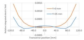
Figure 7: Calculated integrated electrical field uniformity.
