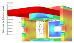
Figure 4: Opera-3D model of half the magnet at 0.12 T. The floating special shaped poles are visible.
