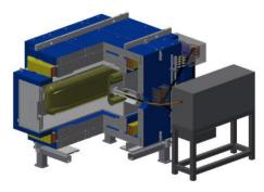
Figure 2: Complete Wien Filter with high voltage supply.
