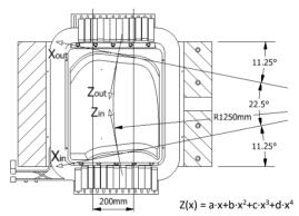
Figure 8: Layout of the B2 dipole with the entrance and exit coordinate system for the fringe field evaluation.
