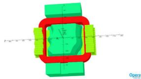
Figure 11: Opera-3D model of the top half of B3.
