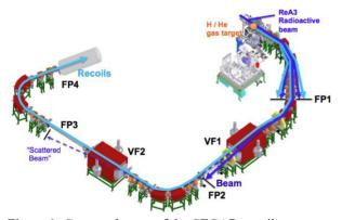
Figure 1: Concept layout of the SECAR recoil separator.
