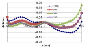
Figure 10: Measured deviations of the effective field boundary as function of horizontal position for the B2 exit end at a range of excitations.
