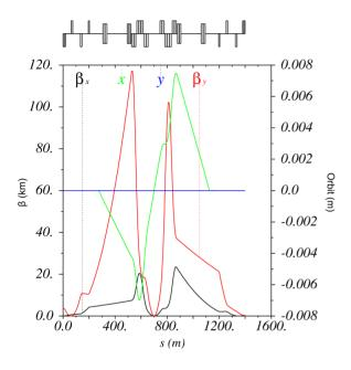
Figure 3: Twis Functions and Orbit for  $0.2 \times 1 \text{ m } \beta^*$  Flat Optics
