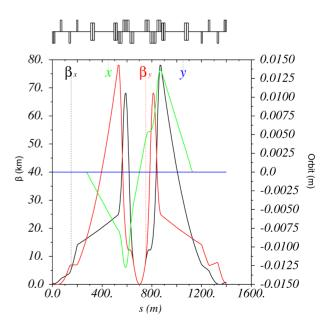
Figure 2: Twis Functions and Obit for 0.3 m  $\beta^*$  Round Optics
