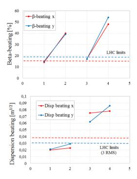
Figure 4: 90-percentile of the residual beta-beating (top) and dispersion beating (bottom), see Fig. 2 for the description of each case studied.
