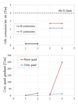
Figure 2: 90-percentile of the integrated strength of the orbit correctors (top) and gradient of the quadrupole correctors (bottom) for the cases at injection with no dipole a2 error (1), at injection with dipole a2 error (2), at collision with no dipole a2 error (3), at collision with dipole a2 error (4).
