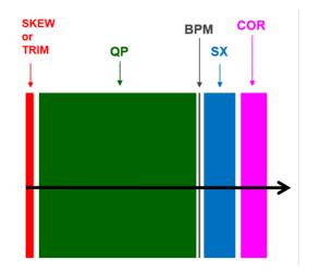
Figure 1: Structure of a quadrupole unit, with from left to right a skew or trim quadrupole, the quadrupole itself, a BPM, a sextupole and an orbit corrector.
