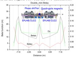
Figure 1:  $\beta$  function for a double mini- $\beta_{\nu}$  lattice.[1,2].
