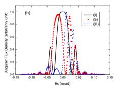
Figure 2: (a) Trajectories in the horizontal plane for electrons of different initial phase space coordinates (i)-(iii). (b) Profiles of the angular radiation distribution as generated by electrons travelling along trajectories corresponding to those in (a). The phase space coordinate (i) represent the on-axis electron and (ii), (iii) is the off-axis electron.
