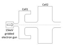
Figure 1: Schematic of Independently-tunable-cells thermionic RF gun (ITC-RF gun)
