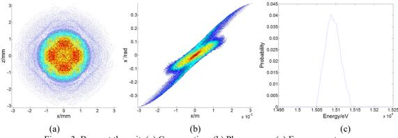
Figure 3: Beam at the exit. (a) Cross section; (b) Phase space; (c) Energy spectrum.
