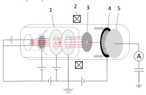
Figure 4: Schematic of test bench. 1 electron gun; 2 FCT; 3 beam scraper; 4 decelerating grid; 5 collector.
