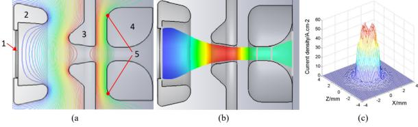
Figure 2: Simulation results of CST. (a) Equipotential line, 1 emitter, 2 focus electrode, 3 intermediate electrode, 4 anode, the maximum electric field occurs at 5; (b) Beam envelop; (c) Current density at the exit.
