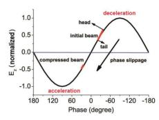
Figure 1: Principle of brake-applied velocity bunching.
