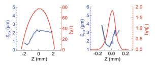
Figure 2: Slice emittance (blue) and current (red) profiles for the uncompressed (left) and compressed (right) beams.
