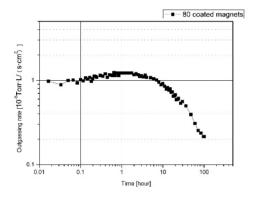
Figure 3: The outgassing rate of the samples.
