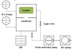
Figure 2: Schematic diagram of the test equipment.
