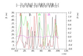
Figure 4: The Twiss function of the transport line starting from the extraction Lambertson.
