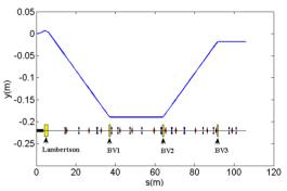
Figure 3: The layout of the two transport line in vertical plane.
