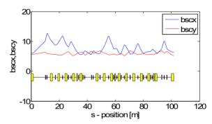
Figure 5: The beam-stay-clear of the transport line.
