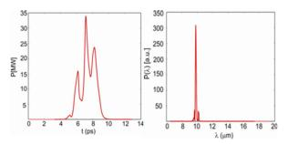
Figure 6: Power distribution along the bunch (left) and the radiation spectrum (right) at the saturation point for radiation wavelength of  $10 \mu m$ .
