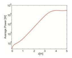
Figure 5: The SASE FEL radiation power along the undulator for 10  $\mu$ m radiation wavelength
