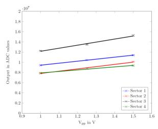
Figure 4: Output as the sum of 4000 events of VELO for three different Peak-to-peak voltages for the R-type sensor.
