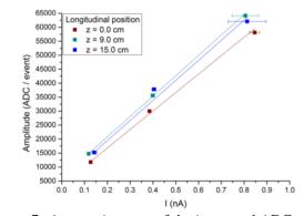
Figure 7: Average increase of the integrated ADC values in the  $\phi$ -sensor No. 76 per readout event versus the proton beam intensity measured by the FC [4].
