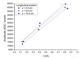
Figure 6: Average increase of the integrated ADC values in the R-sensor per readout event versus the proton beam intensity measured by the FC [4].
