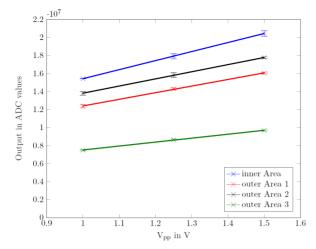
Figure 5: Output as the sum of 4000 events of the VELO for three different Peak-to-peak voltages for the  $\phi$ -type sensor.
