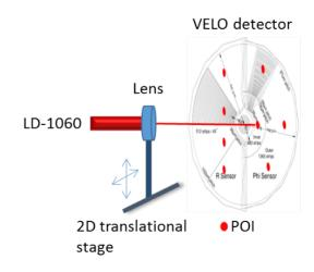
Figure 2: Setup of the LD-1060 to measure the output of the
