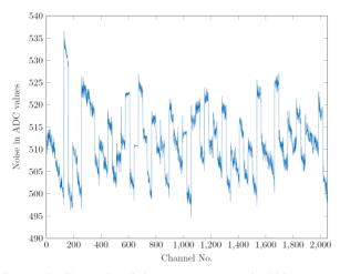
Figure 3: Example of the noise (mean of 4000 events in ADC values) per Channel of the R-type sensor.
